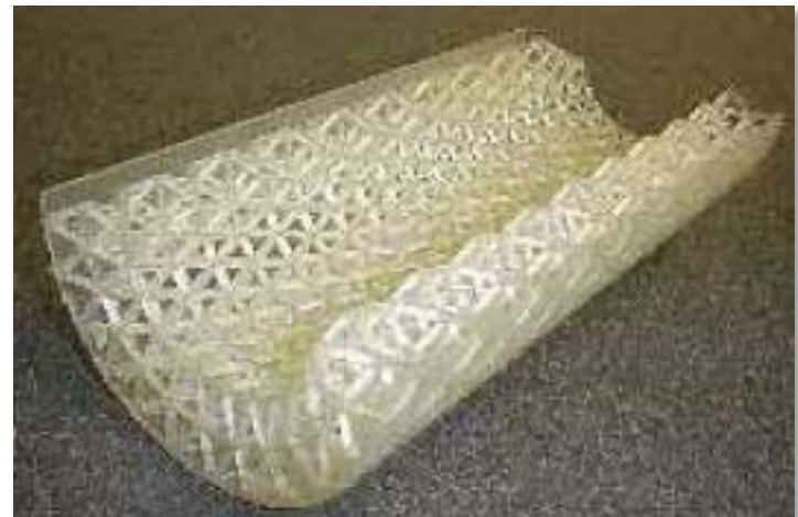
A test part built by SLA
