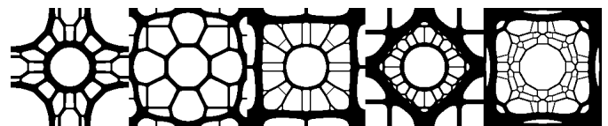
Figure 1: Illustration of poorly connected microstructures. The unit cells are individually optimized for maximum bulk modulus under linearly-varying volume fractions from 30% to 50%, from left to right.
