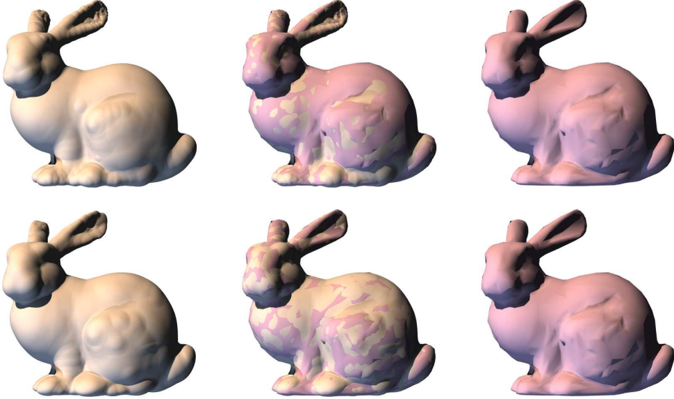
Fig. 3. The reconstructed implicit surfaces using spherical (top left: with 639 blobs, L_{mean} = 0.16 and L_{max} = 0.53 ) and ellipsoidal (bottom left: with 300 blobs, L_{mean} = 0.03 and L_{max} = 0.29 ) blobby objects respectively. The top middle is a superimposed image of the given model and spherical blobs. The bottom middle is an image superimposed with the given model and ellipsoidal blobs. The two right images are the given bunny model.
