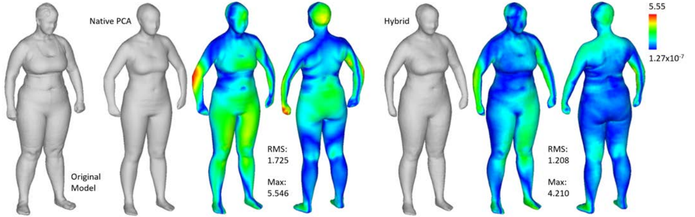
Figure 17: A female model reconstructed by linear regression with 8 parameters – from left to right are the original model, the model generated by native PCA-based representation with 5 PCs and the model generated by hybrid representation with 10 PCs having the same memory consumption. The color maps give the distribution of vertex-to-vertex distance errors (unit: centimetre).
