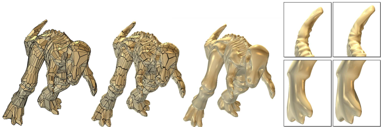
Figure 24: A dinosaur model with 2,382 polygons and 12,146 vertices, where in the zoom-views our results (left) are compared with the PN triangles (right). The unwanted creases shown on the PN triangle model do not appear on our result.
