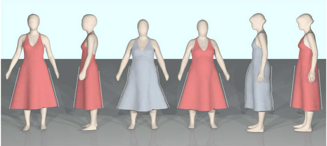
Figure 1: Shape control for the 3D automatic resizing of apparel products can be flexibly performed by specifying features (illustrated by the white dashed curves) on the apparel products. The shape of resized products around the features is processed to match the designed shape. This improves the quality of shape on the results of automatic resizing. From left to right, the designed dress worn on a model, side view of the designed dress, the automatic resizing result without shape control on the features using the method of [Wang et al. 2005], our result with the shape of features preserved, the automatic resizing result without shape control, and our result giving straight profiles as the designed shape of the dress.
