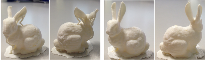
Fig. 7. Physical models fabricated by FDM using MakerBot Replicator 3D printer: (left-two) an original model and (right-two) a model after applying our shape optimization. The supporting structures are generated by MeshMixer.
