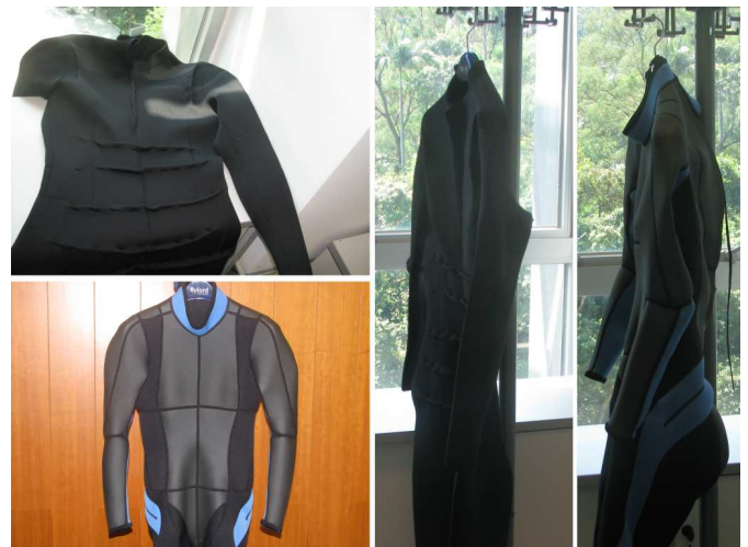
Fig. 2. Wetsuit produced by conventional tailor-making (top-left and middle column) vs. wetsuit fabricated from 2D pieces generated by our system (bottom-left and right column) – it is easy to find that the conventional wetsuit is a planar design but the wetsuit made by our system is a real spatial one.
