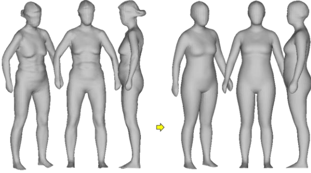
Fig.4. On increasing the bust-girth of a model from 91cm (left) to 99cm (right) – feasible human body can be reconstructed. The computation employs 15 PC coefficients.
