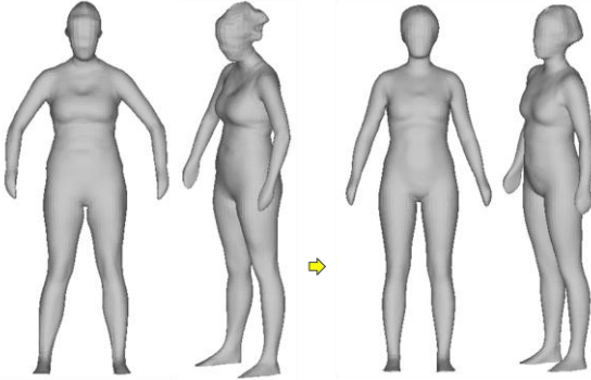
Fig.12. An example of parametric design of human body: to build a model with Height = 174cm, Bust = 93cm, and Waist = 80cm.
