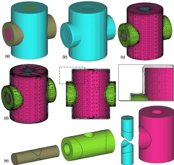
Figure 10: Generating general offset surface on a mechanical part: (a) the hRay-rep of the model, (b) the hRay-rep of the general offset surface, (c) the surfaces generated from hRay-rep – sharp features are well preserved, (d) the meshes for the general offset surface and the mechanical part, and (e) the assembly drawing of homogeneous regions.
