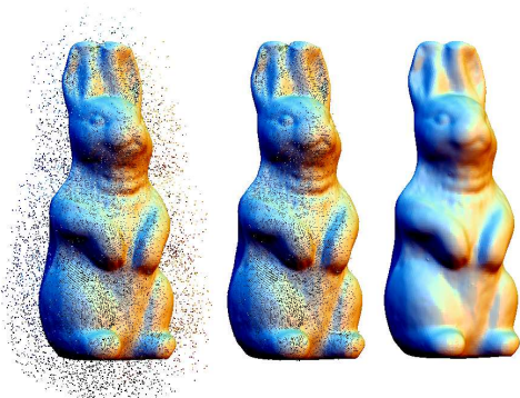
Figure 14: Reconstruction results on a large noisy point set: (left) original noisy points, (middle) the resultant point set after removing outliers [24], (right) result from multi-level quasi-interpolation with an adaptive shape parameter.
