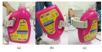
Fig. 14. Caging to grasping process for the detergent container using a soft gripper. The gripper starts to grasp at a place not stable as shown in (a) and will slide while shaking the gripper. Since the detergent has two isolated caging grasps, the soft hand will slide upwards or downwards according to the shaking direction, and eventually reach a stable grasp as (b) or (c).
