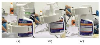
Fig. 13. Caging to grasping process (from left to right) for the spray container using a soft gripper. The grasping starts from a place as shown in (a) which is not stable and will slide upwards while shaking the gripper, and then eventually get immobilized at a stable grasp as (c).
