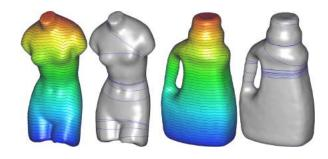
Fig. 6. Local minimal rings generated on two examples: (left) the Venus model with 6.4k vertices – 11 rings are generated, and (right) a container model with 10k vertices — results in 19 curves.
