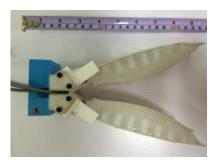
Fig. 12. A soft gripper that can achieve the caging grasp in a way similar to ropes.
