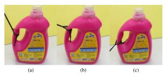
Fig. 11. Caging to grasping process for the detergent container using a rope. The rope starts at a non-stable caging in (a), and then will reach two different stable grasps as shown in (b) and (c), according to whether stretching the rope upwards or downwards.
