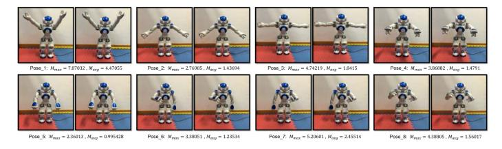
Fig. 6. Eight basic poses are reconstructed by our method (left of each pair) and compared with the ground truth (right of each pair). The similarity metrics,  $M_{max}$  and  $M_{avg}$ , of each pair are also reported. The evaluation is taken on a projection defined by using 1,644 landmark pairs.
