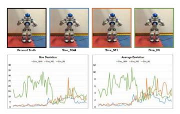
Fig. 8. To reconstruct motion using landmark sets with different number of corresponding samples, statistics of  $M_{max}$  and  $M_{avg}$  in degree indicate that more landmark pairs lead to better results.
