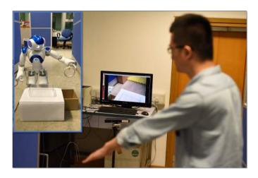
Fig. 1. An example of imitation realized by our framework working with the NAO humanoid.
