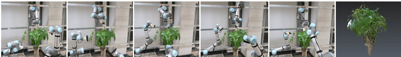
Fig. 5. The progressive views of plant phenotyping by our multi-robot. These pictures are taken when our multi-arm system is running the proposed deep NBV planner. The last column depicts the resultant point cloud of the plant. One can watch the accompanying video for a complete illustration.
