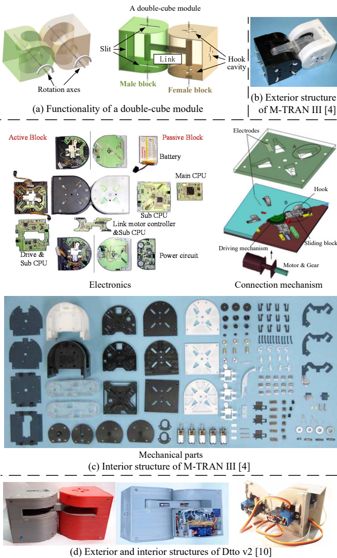
Fig. 1. All self-reconfigurable robots using double-cube modules have similar exterior structures and similar functions that: each module consists of two semi-cylindrical boxes and a link, and each box can rotate independently around its axis by \pm 90^\circ (see (a) for the design of our EasySRRobot). The male box (in green color) has slits on its three faces, and the female box (in yellow color) has hook cavities on its three faces. The double-cube modules used in M-TRAN III (see (b) and (c)) and Dtto v2 (see (d)) have different interior structures for placing on-board components, which lead to different placements of the link – the link of Dtto is placed closer to one side of the box than the other side. M-TRAN photos are courtesy of Prof. Haruhisa Kurokawa.
