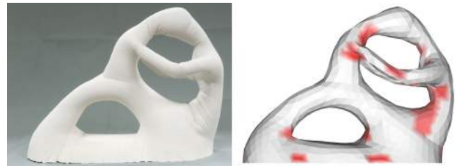
Fig. 16. The location of wrinkles on a fabricated model can be well predicted (red regions in colormap) by analyzing principal stretch values.
