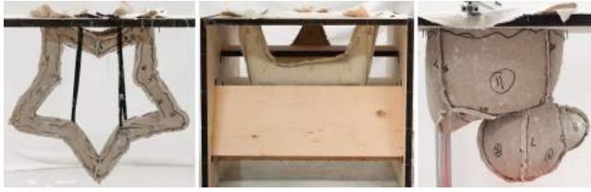
Fig. 13. Fabric formwork. (Left) Star model with four string supports. (Middle) Chair model with four planes. (Right) Duck model with a cable and a string support.
