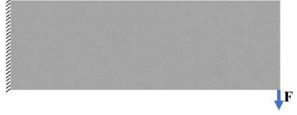
Fig. 3 The design domain and boundary conditions. The design domain is discretized into 120 \times 40 square bilinear finite elements.
