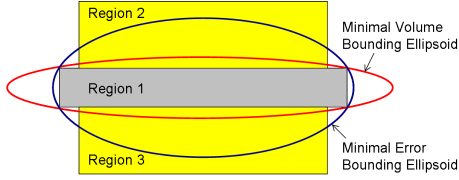
Figure 2: The minimal volume bounding ellipsoid (MVE) in general is not a minimal error bounding ellipsoid (MEE) in terms of the shape and solid approximations. To construct the bounding ellipsoid for the gray region, the MVE yields both the greater shape approximation error and the greater volume approximation error to the given model M consists of 3 regions. MEE gives a better approximation to M although its approximation to region 1 is not as good as MVE.
