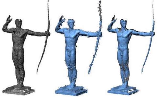
Figure 13: Reconstructions from an input with noises and outliers: (left) input point cloud, (middle) the reconstructed surface before post-processing and (right) the resultant surface after mesh cleaning.
