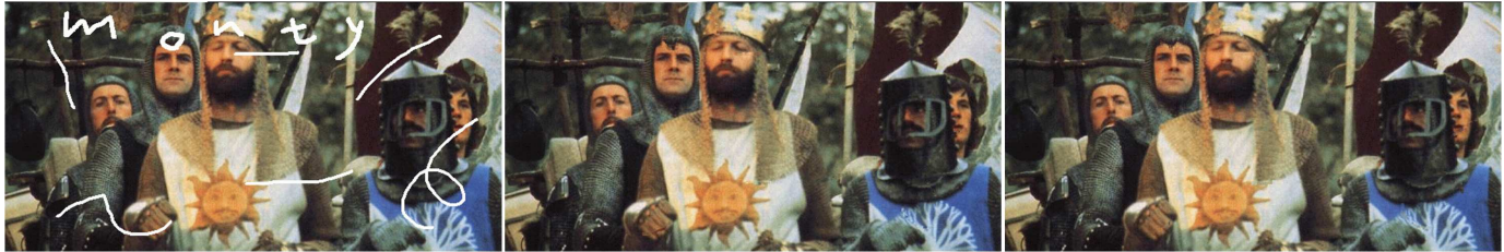
Fig. 7. An example of removing the unwanted drawing: (left) the input image with annoying drawing ( 628 \times 316 pixels), (middle) the result of Criminisi's method (in 47.14 sec.), and (right) our result (in 3.68 sec.).
