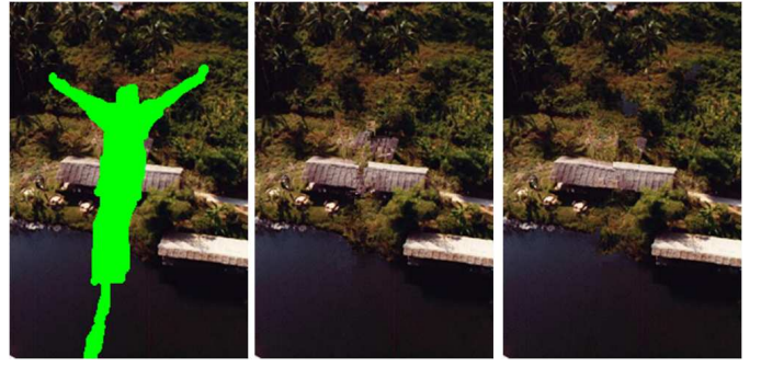
Fig. 4. An example of removing a bungee jumping man: (left) the input image ( 206 \times 308 pixels), (middle) the result of Criminisi's method (in 12.5 sec.), and (right) our result (in 0.9 sec.).
